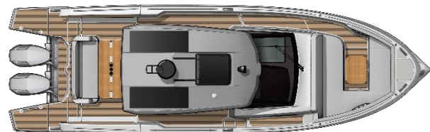
Hard top - Solar panels
